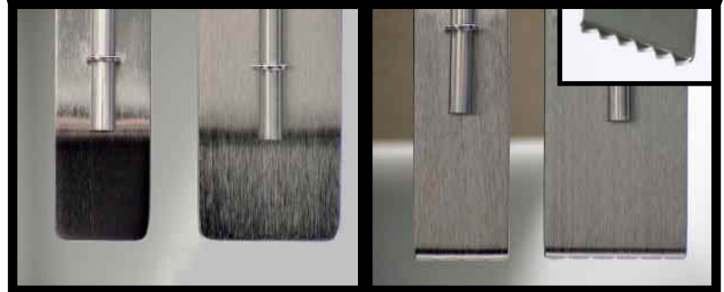
Blades can have a smooth finish with 15° angled tip or can have a sharp 90° angled saw toothed end.
